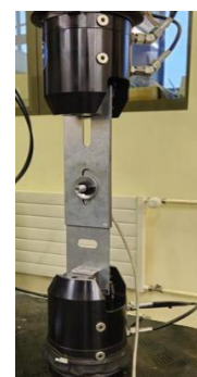
Fig. 5 Walter & Bai servohydraulic testing machine.
