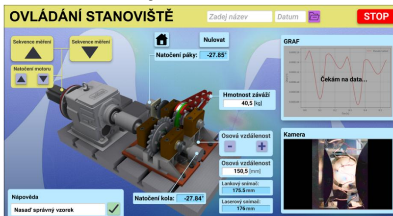
Fig. 1 GUI - control system of the test rig
