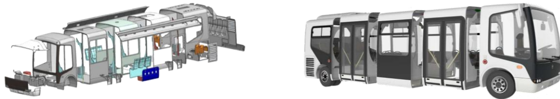
Fig. 1 Modular composite structure and monocoque bus design.
